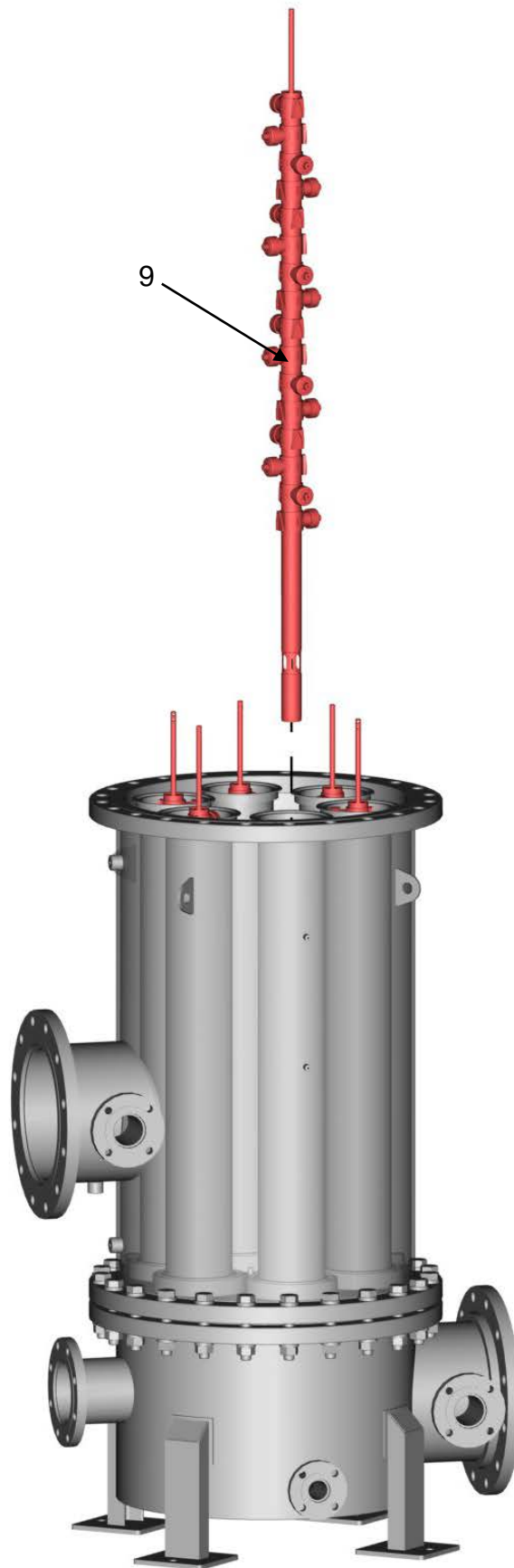
Figure 13 - Suction Scanner Removal
