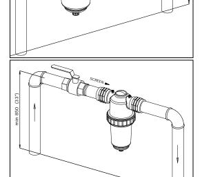
Maximum pressure drop across the filter element, for a short time should not exceed 1 bar (14 psi).
