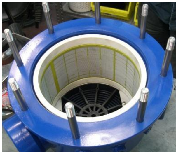
Screen Seated Properly
