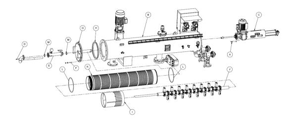
Opening the filter and disassembling its inner components is necessary for changing screens, periodic maintenance and repairs. Prior to opening the filter it is recommended to operate a flushing cycle.
